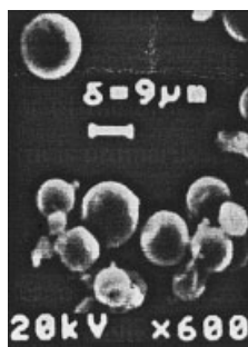
Figure 2 Morphology of G-PDLLA-MS by SEM.
